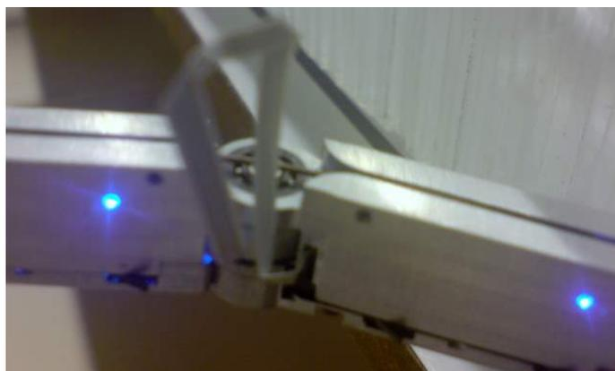
Figure 3.20: Two segments with continuously lighting LED's. This indicates that at some point the angle sensor did not provide a valid angle measurement. If an LED is lighting after an experiment, then this suggests that data is partially bad.
