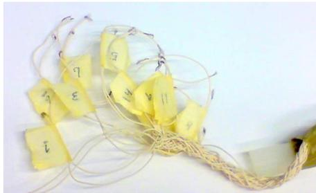
Figure 3.8: Using a bus architecture prevents the accumulation of wires as new sensors are added. This is the base connection of an antenna with a series of flex sensors.
