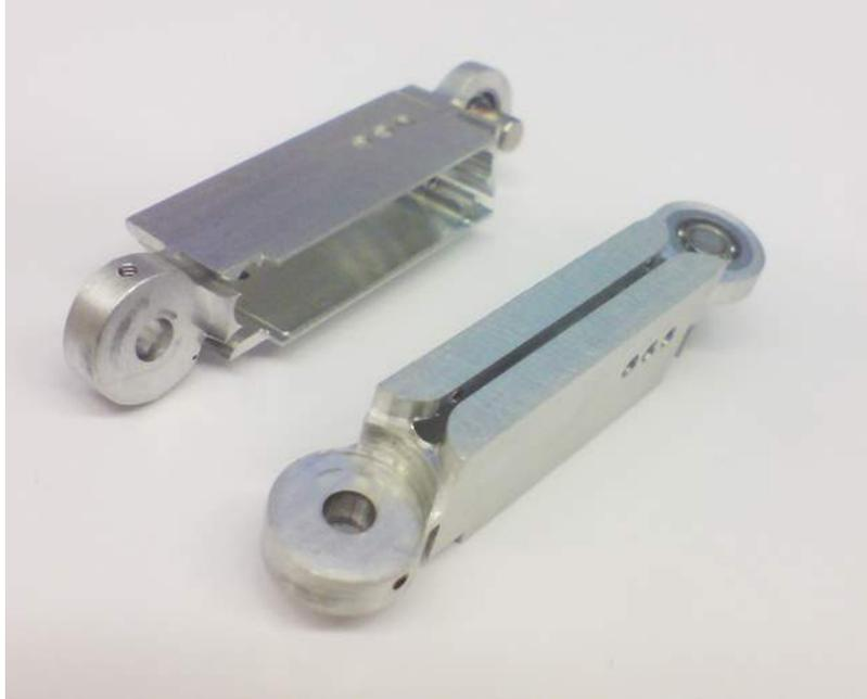
Figure 3.9: The top piece of the designed aluminum shell.
