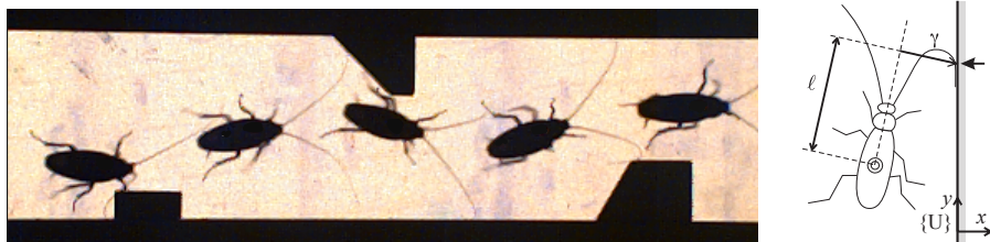
Fig. 11. Left: Multiple exposures of the cockroach P. americana negotiating a set of obstacles at high speed, using feedback from its antennae [6]. Right: A simplified model of an antenna as a distance-to-wall sensor.
