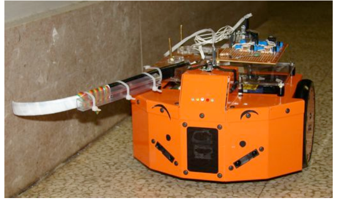
Fig. 6. The cast urethane antenna with embedded flex sensors mounted on the Garcia robot.
