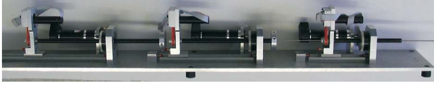
Fig. 3. Three-tube, six-DOF active cannula actuation unit used in experiments.
