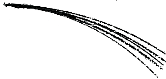
Figure 3.15: The final needle locations, extracted from difference images, with different bevel angles illustrate the steering effect of the bevel tip. A 5° bevel exhibits the most bending while an 80° bevel exhibits the least.
