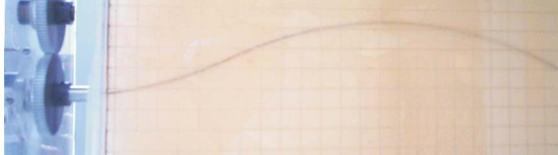
Figure 3.20: (Top) The bicycle nonholonomic model prediction for a run with two curves, shown with average data (including nuisance parameters) and standard deviation bars. (Bottom) During the experiment, the needle was inserted 8.3 cm, spun 180^\circ , then inserted another 16.7 cm.
