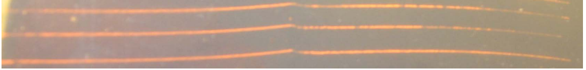
Figure 3.30: Trajectories cut through Supersoft Plastic phantom tissue, after needle withdrawal (and corresponding tissue relaxation). Note the kink near the middle of the runs, where the needle was rotated 180^\circ .
