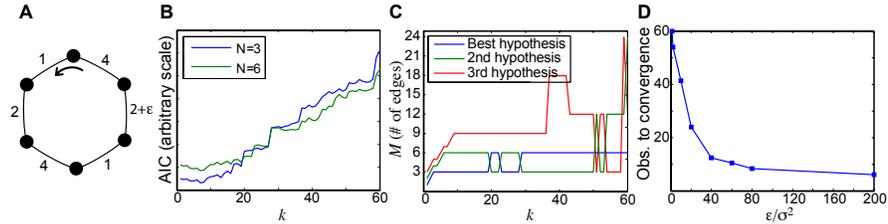
Fig. 5: An illustration of loop re-opening using the AIC model selection criterion. A: The simple (but almost ambiguous) map given to the robot. B: The AIC of the hypotheses for a 3-edge and 6-edge cycle evolving over time. C: The top three hypotheses at any period during the same trial. D: The average convergence time to the correct hypothesis as a function of  $\varepsilon/\sigma^2$ .
