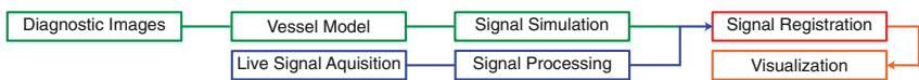
Fig. 1. In Bioelectric Navigation, live bioelectric measurements are registered to simulated signals from a pre-interventional image to identify the catheter's position.
