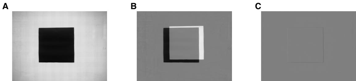
Figure 6.8: (A) Three translational DOFs goal image. (B) Difference between the goal and the initial displacement images. (C) Difference between the goal and the final images.
