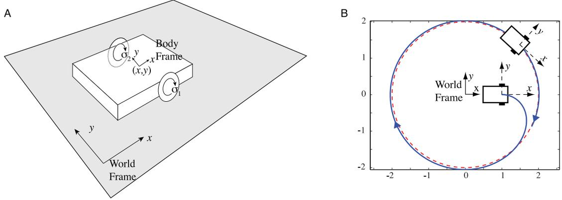
Figure 5.4: (A) Differential drive robot. World and body reference frames are shown. The body frame's  $x$ -axis is along the forward translational velocity of the robot. (B) Differential drive robot following a circle. Dashed circle is the desired circle to be followed by the differential drive robot. Initially the robot is away from the desired circle but with the application of the controller, it follows the circle. Axis scales are dimensionless for purposes of demonstration.
