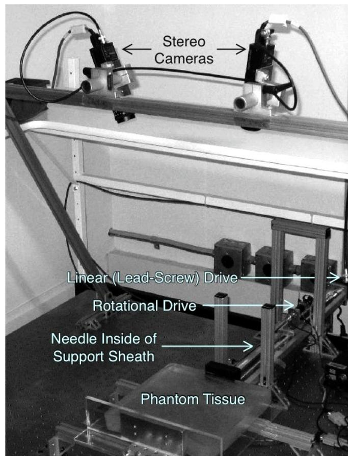
Figure 2.2: The needle steering device inserts the needle into the tissue phantom while the needle tip position is tracked using two overhead stereo cameras.
