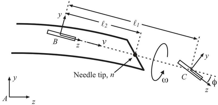
Figure 2.3: Kinematic generalized bicycle model: Frame  $A$  is the inertial world reference frame. Frames  $B$  and  $C$  are attached to the two wheels of the bicycle. This figure is reproduced from [85] with permission from the authors.
