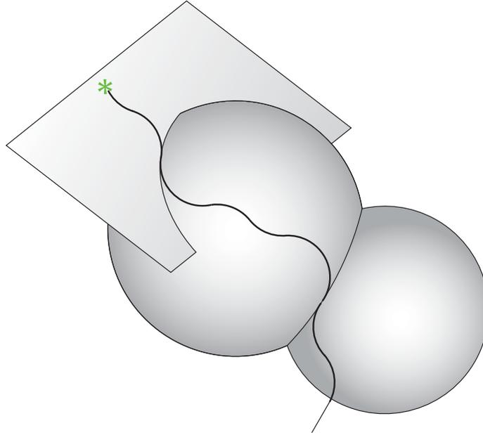
Figure 3.2: A stylized depiction of a needle trajectory that remains within a sequence of 2D patches. The plane-following controller was reported in Section 3.1, and the sphere-following problem is reported in Section 5.4.2.
