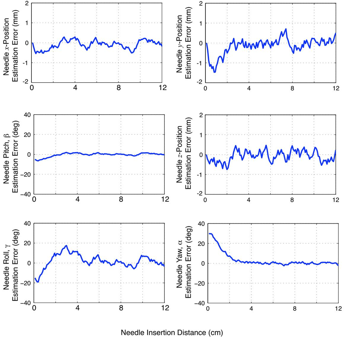
Figure 4.4: Asymptotic observer to estimate the full 6-DOF pose of needle steering from just the position measurements in MATLAB simulations. The radius of curvature of the needle in the tissue is taken as 12.2cm. Noisy needle tip position data is collected every 1mm of insertion, with measurement noise that is uniformly distributed within  $\pm 1$ mm. The estimation errors converge to zero in all the six degrees of freedom with a low steady-state variance.
