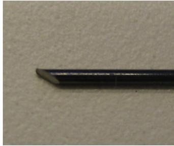
Figure 2.1: Flexible bevel-tip needle. As the needle is inserted into tissue, the asymmetry of the bevel creates a moment at the needle tip, deflecting the needle and causing it to follow a circular arc. As the needle base is rotated, the bevel tip is reoriented in space, so that subsequent insertion follows another circular arc.
