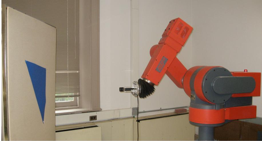
Figure 6.1: Experimental configuration. Camera is mounted on a 6-DOF industrial robot. The camera is looking at a planar scene in front of it.
