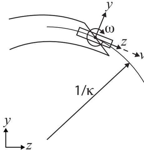
Figure 2.4: Kinematic generalized unicycle model of needle steering. This is same as the generalized bicycle model in Figure 2.3 with  $l_2 = 0$  and keeping  $l_1$  and  $\phi$ . The curvature of the path the needle follows inside the tissue is given by  $\kappa = \tan \phi / l_1$ . This figure is reproduced from [85] with permission from the authors.
