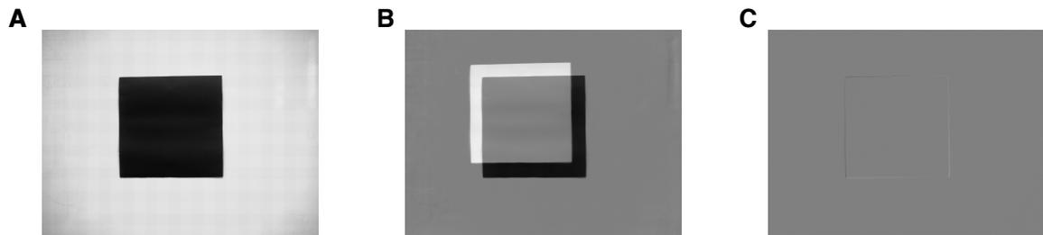
Figure 6.2: (A) 2D goal image. (B) Difference between the goal and the initial displacement images. (C) Difference between the goal and the final images.
