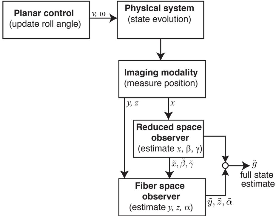
Figure 4.2: Coupled reduced space and fiber space asymptotic observers. The reduced space observer estimates  $x$ -position, pitch and roll of the needle tip from (noisy)  $x$  measurements. The fiber space observer uses these estimates along with the (noisy)  $y$  and  $z$  measurements and estimates the rest of the states of the needle.
