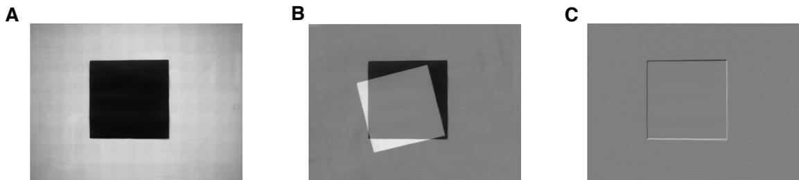
Figure 6.10: (A) SE(2) and depth goal image. (B) Difference between the goal and the initial displacement images. (C) Difference between the goal and the final images.
