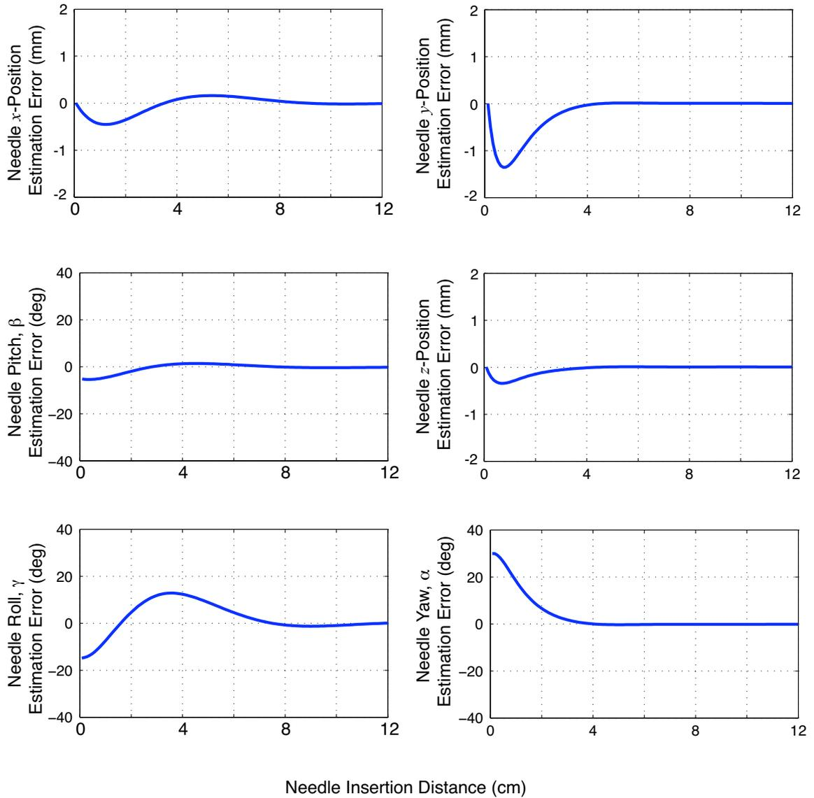
Figure 4.3: Asymptotic observer to estimate the full 6-DOF pose of needle steering from just the position measurements in MATLAB simulations. The radius of curvature of the needle in the tissue is taken as 12.2cm, tip position data is collected every 1mm of insertion with no measurement noise. The estimation errors converge to zero in all the six degrees of freedom.
