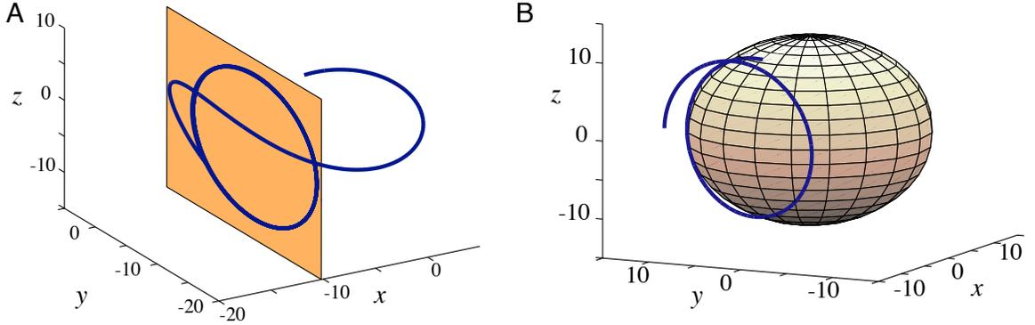
Figure 5.3: (A) Needle tip driven so that at needle tip trajectory becomes parallel to the  $y$ - $z$  plane. (B) Needle tip driven to the desired sphere. Initially the needle tip is away from the desired sphere (drawn in the figure) but with the application of the controller, it converges to the surface of the sphere. Axis scales are in cm.
