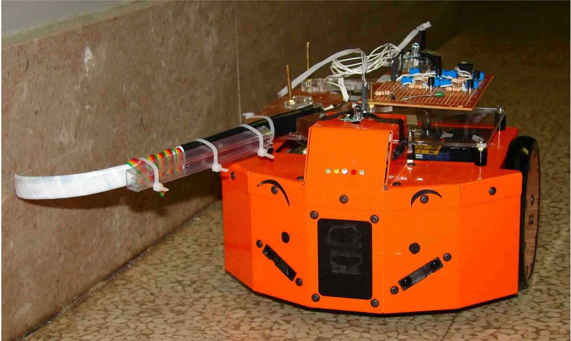
Figure 5.2: The cast urethane antenna with embedded flex sensors mounted on the Garcia robot.
