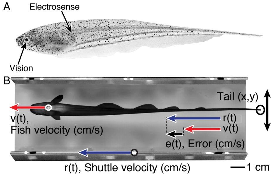
**Figure 4.1 Schematics of *Eigenmannia* and refuge tracking experimental setup**
