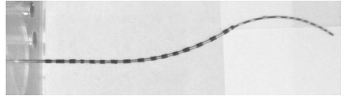
Fig. 10. Experimental photograph from one of the stereo cameras showing the cannula with fiducial markers.
