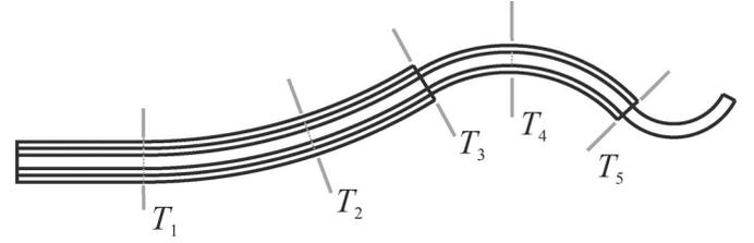
Fig. 4. “Links” or regions of unique overlap of a three-tube cannula composed of tubes like those in the upper image of Fig. 5. Links start and end at transition points, and the  $j$ th link is between  $T_j$  and  $T_{j+1}$ . In this configuration, the largest tube transitions from straight to the left of  $T_1$  to curved to the right. The same is true of the middle tube at  $T_2$  and the smallest tube at  $T_4$ .
