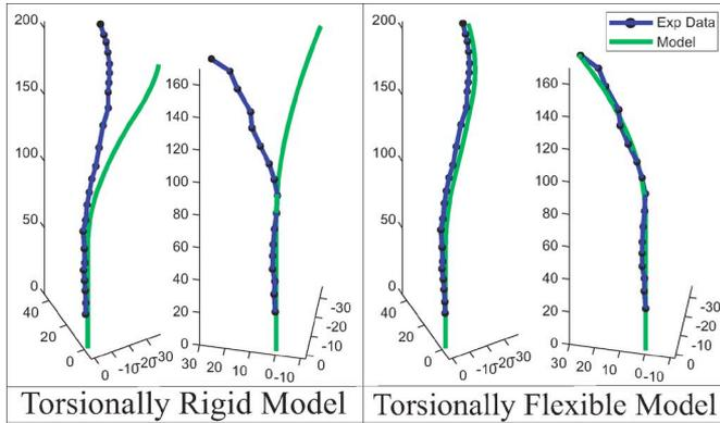
Fig. 11. Experimental data and model predictions of the partial and full overlap conditions at the final input angles before bifurcation ( $200^\circ$  and  $280^\circ$ , respectively). Note that these are also the input angles with the greatest overall tip error for each case. These results show that torsion is a vital part of an accurate active cannula kinematic model.
