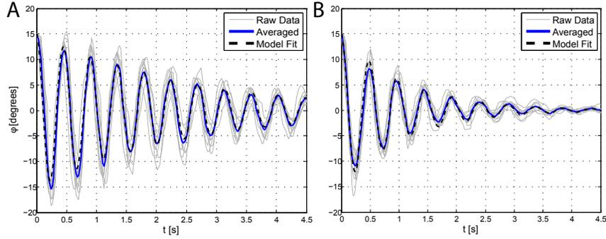
Fig. 3. Pitch angle versus time after pitch perturbations, where the quadrotor propeller gains were “de-tuned” so that pitch was stable but highly oscillatory. **(A)** The open loop (no abdominal control—the abdominal servo-angle is held fixed). **(B)** The servo is controlled in closed-loop via the simple PD scheme described controller (1).
