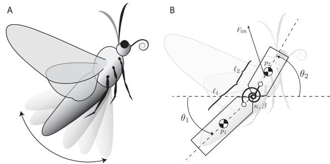
Fig. 1. **(A)** The abdomen of a moth comprises 50% of the mass of the animal. It was recently discovered that strong visually mediated abdominal reflexes of the moth may serve to redirect flight forces for control.<sup>4,6</sup> **(B)** A two-link rigid-body model of sagittal plane dynamics can be used to describe how rapid adjustments of the thoracic abdominal angle, namely  $\theta_2 - \theta_1$ , can be used to redirect wing forces for control.
