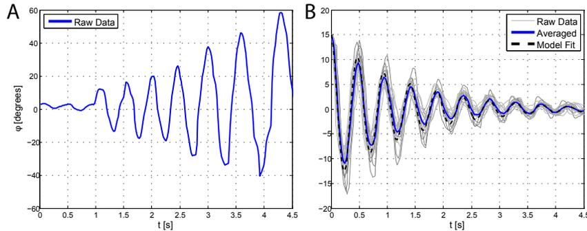
Fig. 4. Pitch angle versus time after pitch perturbations, where the quadrotor propeller gains were “de-tuned” so that pitch was unstable. (A) Response with no abdominal control. (B) Response with abdominal control.
