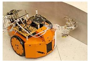
Inspired by cockroach biology, engineers build an antenna for a robot that enables it to scurry along walls, turn corners, and avoid obstacles—just like the insect.
